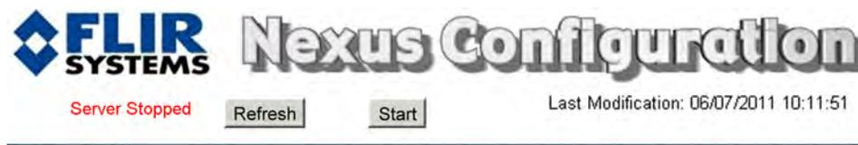
Click on the Start button to restart the server, and when the page refreshes, the status will again show as “Server Running...”. The Start button will be replaced by a Stop button when the startup procedure has completed.
