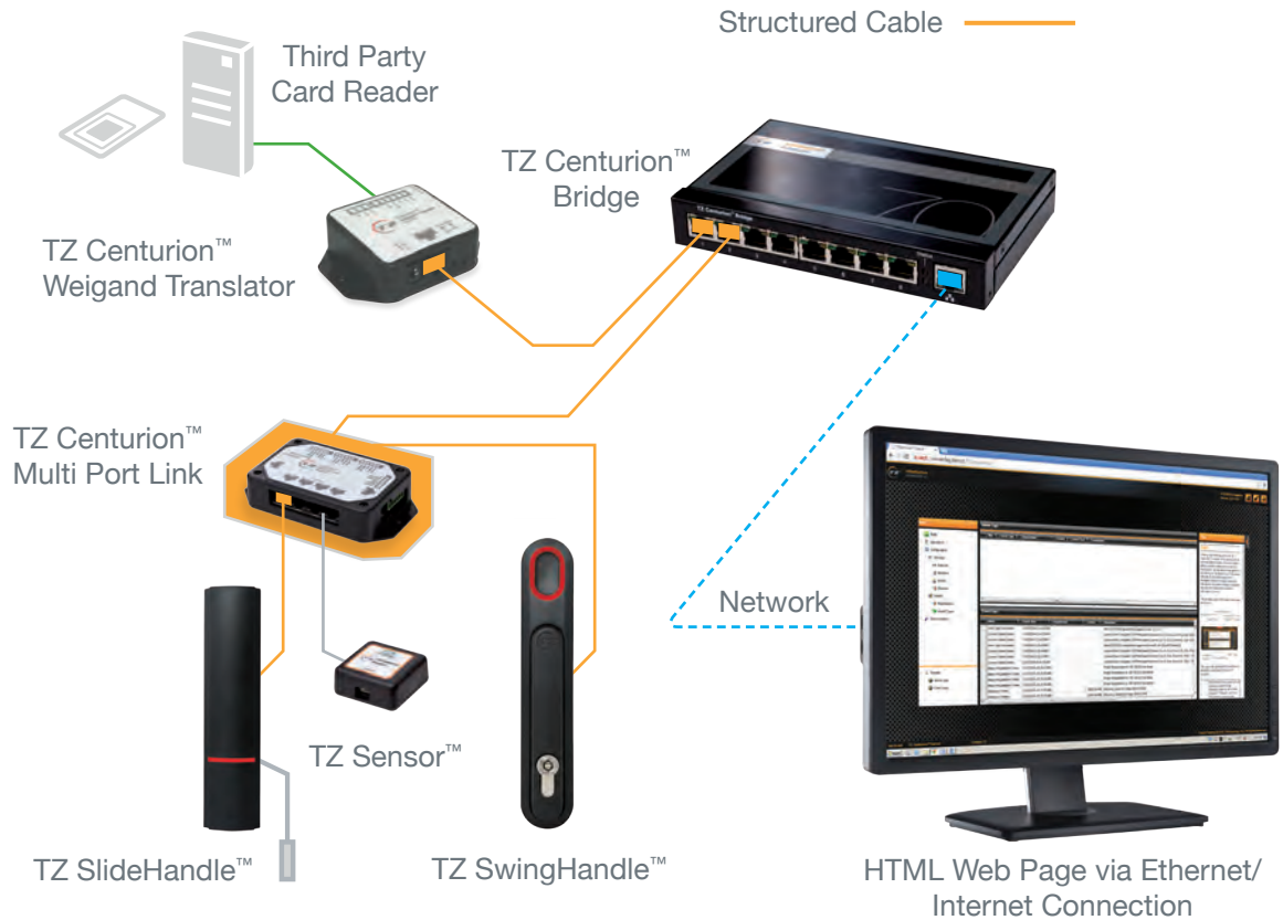
Figure 3: TZ Centurion™ Multi Port Link in a TZ Centurion™ System
