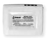
The Model D-67 1-channel Receiver is designed for use in security systems and remote switching functions. Typical applications for the receiver include adding a wireless zone, a panic button, or creating a remote arm/disarm feature for a hardwired alarm panel. Each time a transmitter is triggered with a digital code matching the receiver's digital code, the receiver's relay will activate for four seconds.
