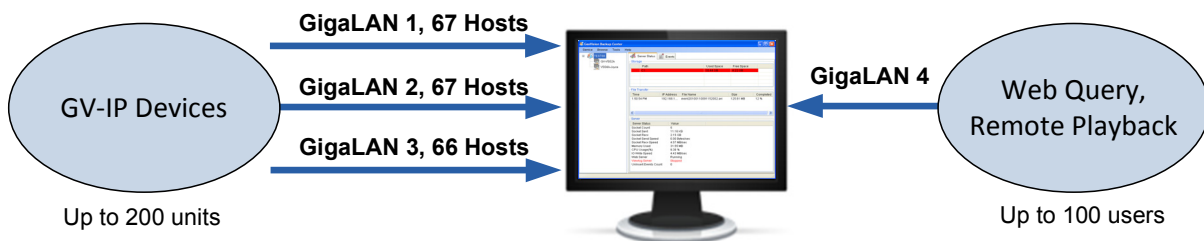
Server installed with GV-Backup Center + 4 Network Cards assigned on different networks
