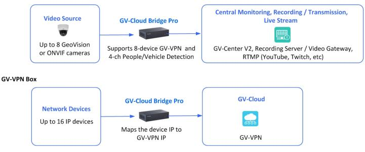
Note: The 4-ch People/Vehicle Detection by GV-Cloud Bridge Pro only works with GV-Center V2 V20.
