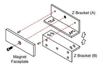
Place Z bracket (A) with the magnet faceplate on Z bracket (B) and insert the supplied M5 (5 mm) screws. Before tightening the screws, adjust the position of the Z brackets so that the magnet faceplate contacts the lock body.
