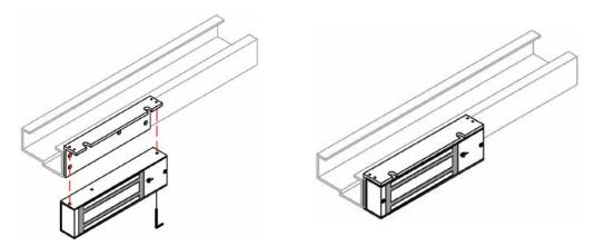
5. Place the two aluminum plugs back into the mounting screw holes.
