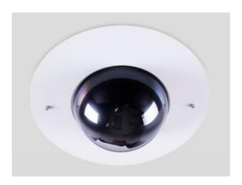
This installation method is only applicable to **outdoor GV-IP Speed Dome** (**GV-SD220-S**). The complete installation weights 6.75 Kg / 14.88 lb. Make sure the chosen ceiling can bear the weight.
