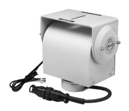
The **PT280-24P** is a "mini" light duty, indoor pan/tilt that is factory prewired for feedthrough of all control functions (pan/tilt, motorized zoomlens, 24 VAC camera power, and video). All connections are made at the input connector, eliminating the need for wiring harnesses made in the field. This feature greatly reduces installation time, while increasing the reliability and serviceability of the system.
