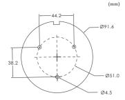
④ Route and connect the cables. Then secure the mounting base to the ceiling or wall with the screws provided.
