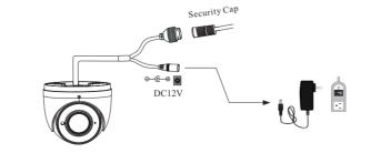
\* 1 It is recommended to install the security cap for outdoor installation.
