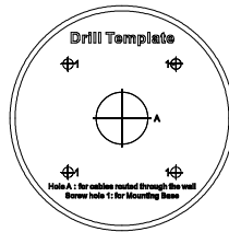
Figure 2-9 Drill Template of the Junction Box
