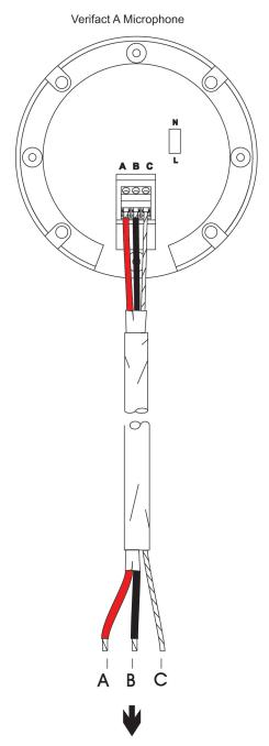
To Louroe Base Stations and Audio Interfaces or Line Level Audio Receivers
