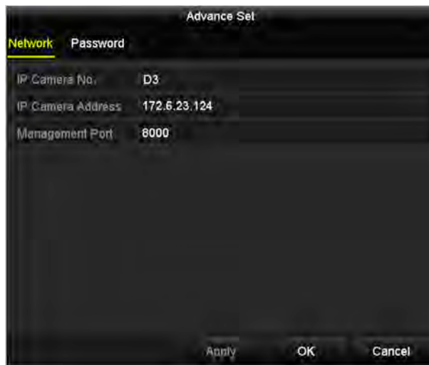
Figure 2. 25 Network Configuration of the Camera
