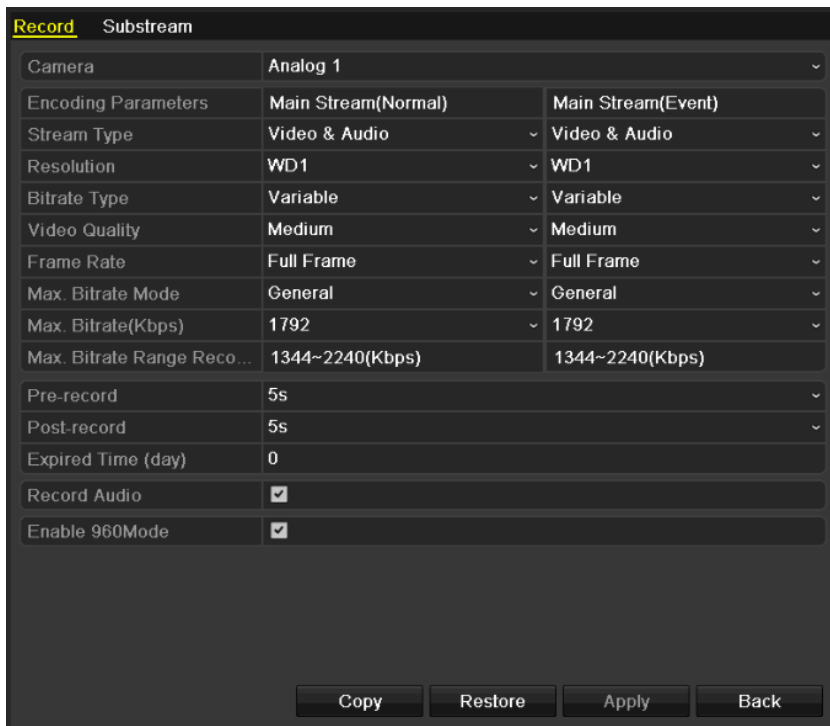
Figure 5.3 Encoding Parameters-Main Stream
